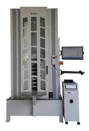
Automatic spring tester AFP-20 static and dynamic tests with servo motor available with specified load ranges:
